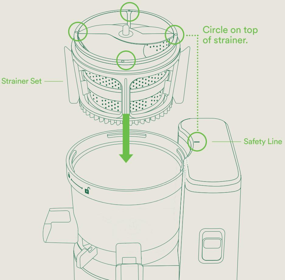
(A) Assemble the hopper with either safety line aligned with
